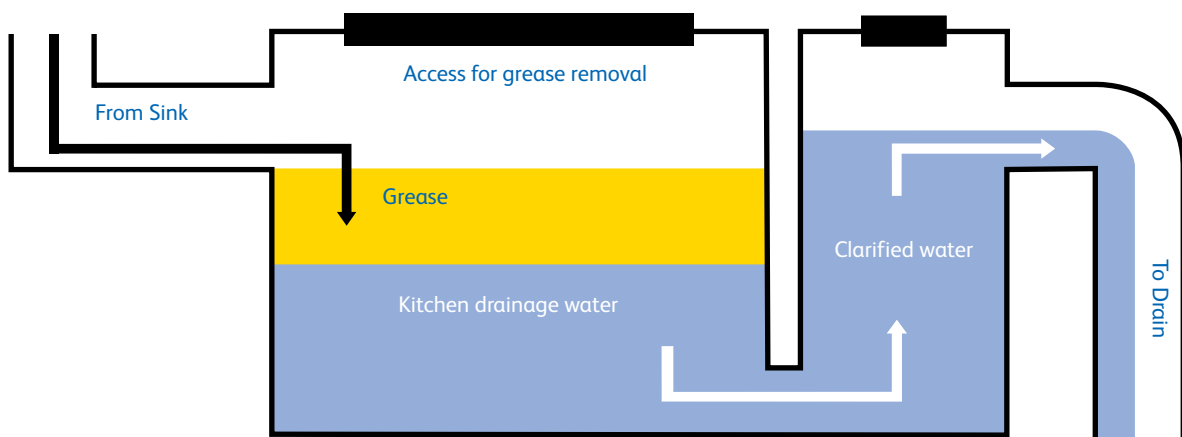
Diagram of an “under-the-sink” grease trap
